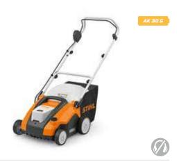
Compact battery aerator for scarifying and combing smaller areas of lawn. Central adjustment of the working depth by means of a rotary switch on the housing, handlebar with 4-setting height adjustment, 34 cm working width, 16 blades. Including an aerator roller and 50-litre grass catcher.
